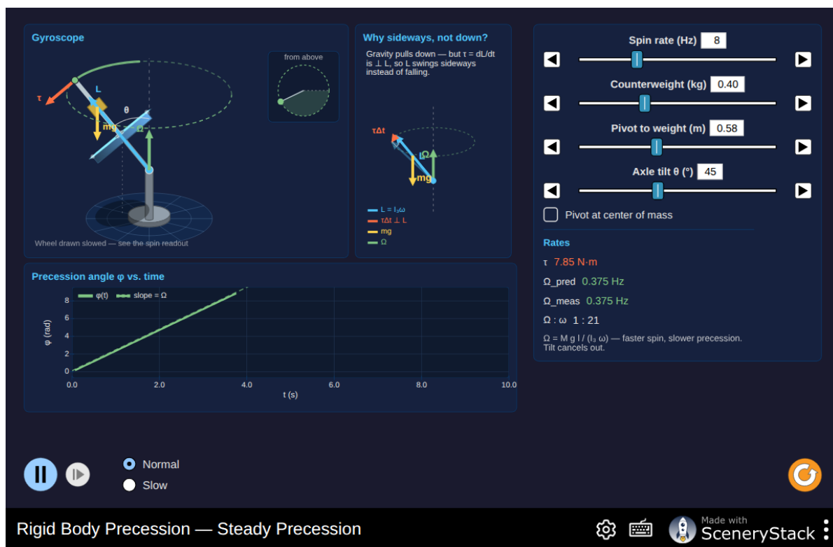
Figure 4.4: A spinning top under gravity, precessing steadily about the vertical. |\vec{L}| and L_z stay fixed while L_x and L_y trace out a circle—the classical motion behind the Bloch vector’s rotation above, and behind the orbital-angular-momentum vector model of Chapter 9. Interactive simulation: Precession
