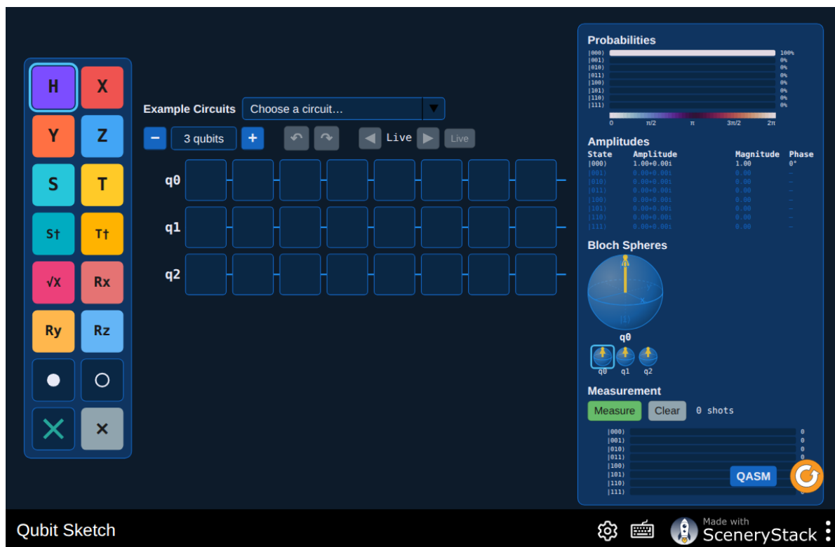
Figure 12.1: Drag X , Z , H , and S gates onto a single qubit and watch its Bloch sphere and amplitudes \alpha, \beta update after each one—the same circuit builder used in Chapter 5 to entangle two qubits, now applied one gate at a time to a single qubit’s state. Interactive simulation: Qubit Sketch
