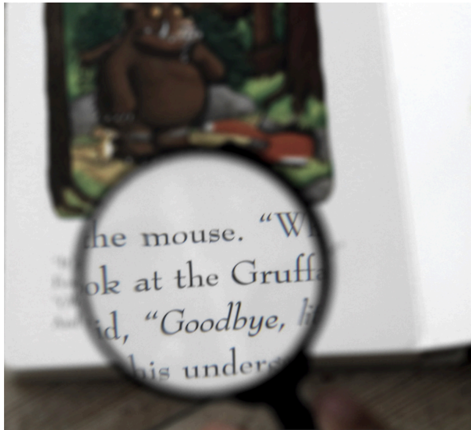
Figure 10: Example of a positive lens used as a magnifying glass (picture taken by A.J.L. Adam / CC-BY-SA 4.0).
