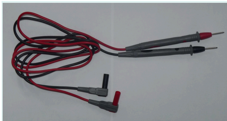
Figure 3.1. These leads used to connect test equipment to circuits in a laboratory are a very rudimentary form of transmission line, suitable only for very low frequencies.
